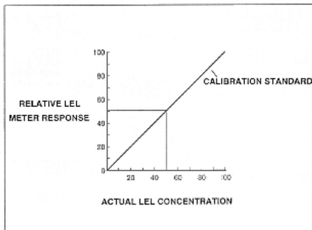
**Figure 1.0: Linear response to the gas used in calibration**
