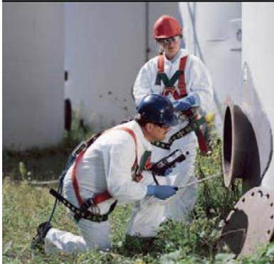
Conditions can change rapidly for many reasons and it is imperative that at least one worker carry and understand the usage of an instrument to monitor for changes in the atmosphere at all times. Even when ventilation equipment is used to purge the air, hazardous atmospheres can exist in ‘voids’ and low lying areas where the air exchange may not be sufficient.
