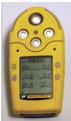
Commonly encountered substances that degrade LEL sensor performance include silicones, lead containing compounds (especially tetraethyl lead), sulfur containing compounds, substances containing phosphorus and halogenated hydrocarbons.
