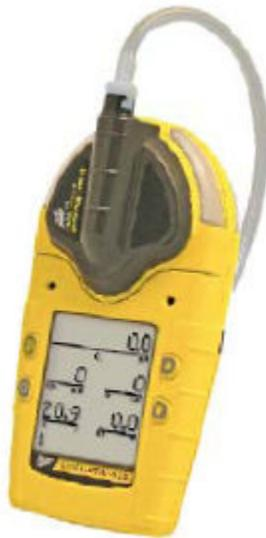
phosphine, hydrogen, hydrogen cyanide, nitrogen dioxide, nitric oxide, chlorine dioxide, ethylene dioxide, ozone and more. Although some of these sensors are cross sensitive to other substances, there is very little ambiguity when it comes to interpreting readings. When you are interested in hydrogen sulphide, you use a hydrogen sulphide sensor. When you are interested in phosphine, you use a phosphine sensor. In many cases, however, a substance-specific sensor may not be available.
